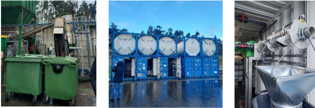
Figure 5: the microAD unit: pretreatment unit (left), digesters (centre), and digestate phase separation (right)
